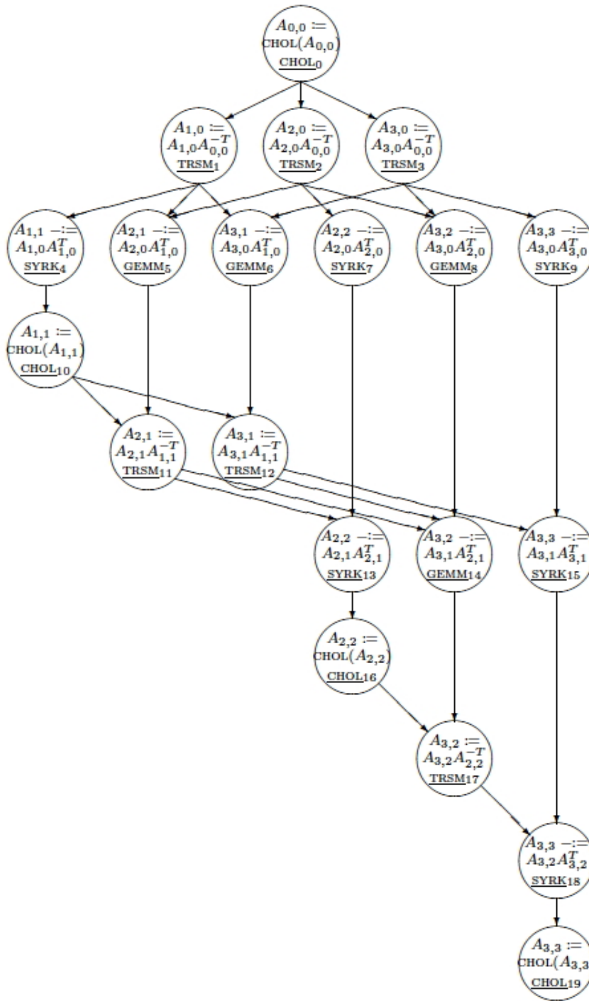
Figure 6.10: Graph of task dependencies in a 4 \times 4 Cholesky factorization
